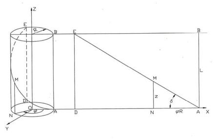
Figure 7. Isometric projection of blade line EMA on vertical plane
