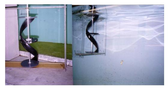
Figure 5. Single Helix Turbine tested at Northeastern University (Photo by B. Gorbaty, 2005)
