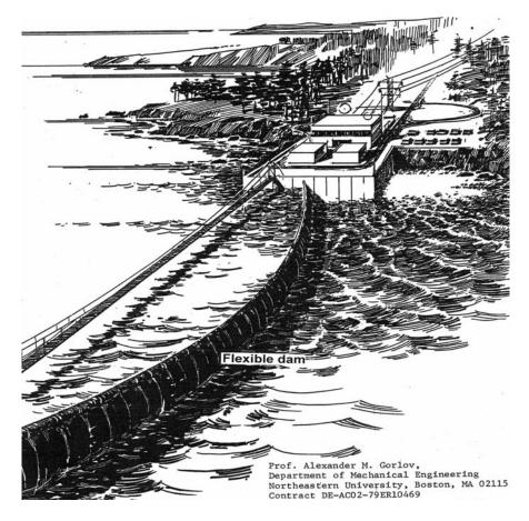
Figure 10. Flexible Barrier for Tidal Power Station (Artistic Rendering, 1981)
