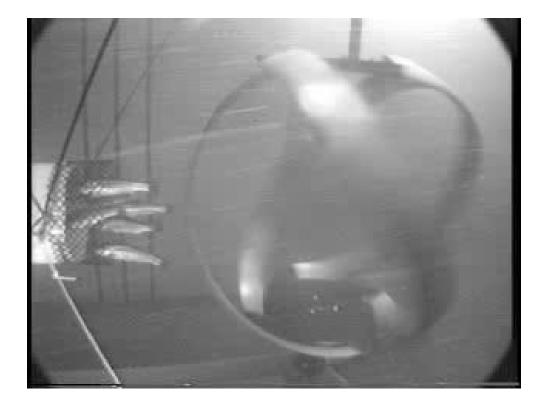
Figure 8. Test with Fish and Spherical Turbine. Water jet direction - from left to right. Courtesy of Alden Lab, 2010
