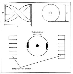
The helical turbine consists of long blades running along a cylindrical surface like a screw thread. The blades provide a reaction thrust from flows in either direction. The design of the turbine allows the engineer to reduce diameter D while increasing its length without power losses, providing important benefits in design.
