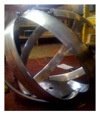
Figure 9. Lucid Spherical Turbine as tested
