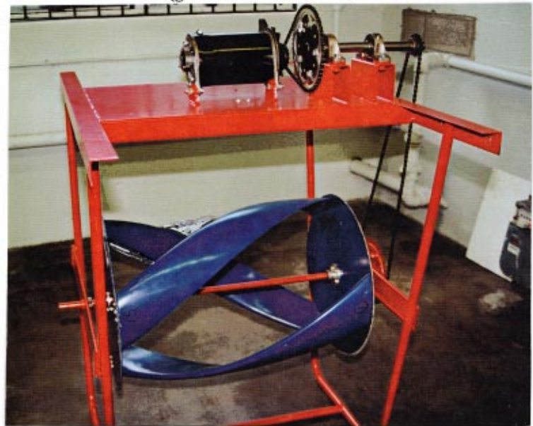
Triple-Helix Turbine (generator above water)
